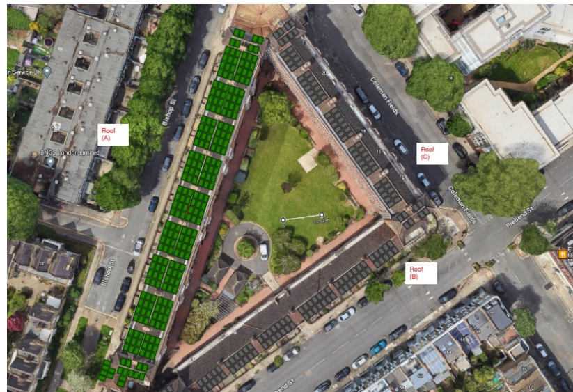
Maximum PV array highlighted in green for the block modelled (pitched roof arrangement at 30 degrees tilt)
